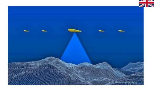
**DESCRIPTION:** The company ABYSSA SAS and its two subsidiaries in the Pacific (in New Caledonia and the Pacific) have developed a design of autonomous deep submergence vehicles using Autonomous Underwater Vehicles (AUVs), navigating as a coordinated fleet in deep water (down to 6,000 meters).
